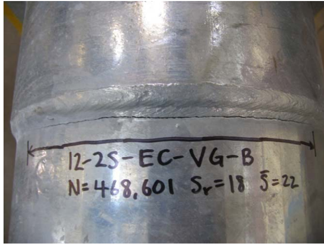
Figure 4-7: Typical External Collar Failure
